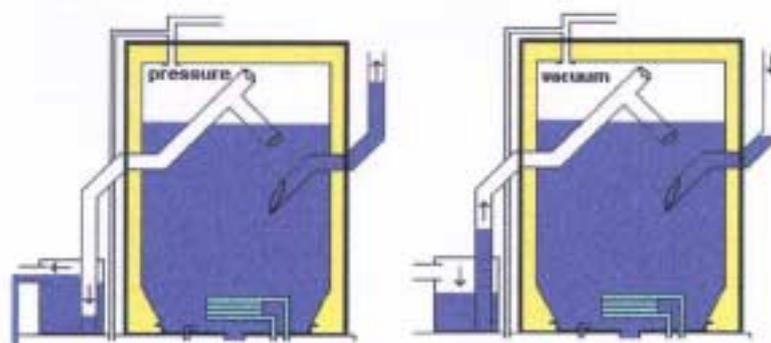
**Figure 3 The first digester is showing the effects of pressure on the system. This situation can occur when gas pressure builds up in the system. The second digester is showing the effects of vacuum on the system. This occurs when the solids valve is opened.**
