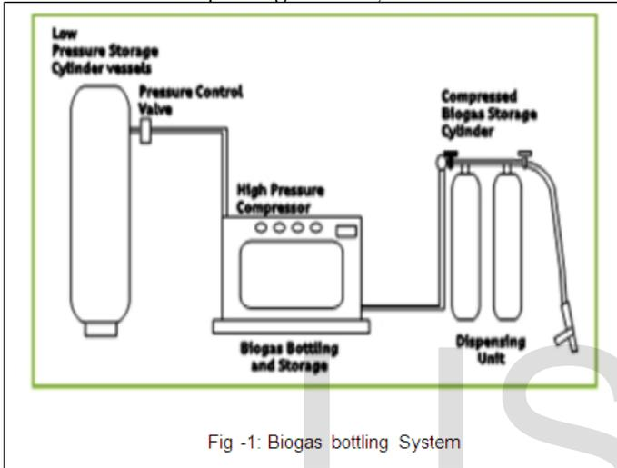
Indian Institute of Technology, Delhi(IIT-D), has developed a small-scale biogas upgrading system using water scrubbing technology (20 m<sup>3</sup>/h system). The water-scrubbing-based biogas up gradation and compression/bottling system is patented IIT-D for enhancing the utility of biogas application that is, in vehicles and cooking applications. The system consists of a water scrubbing column and a methane-enriched biogas compression system.
