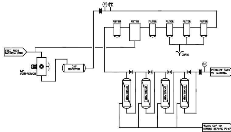
Figure 1. Schematic diagram of the pilot plant
