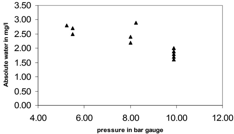
Figure 3. Water content as a function of the operating pressure
