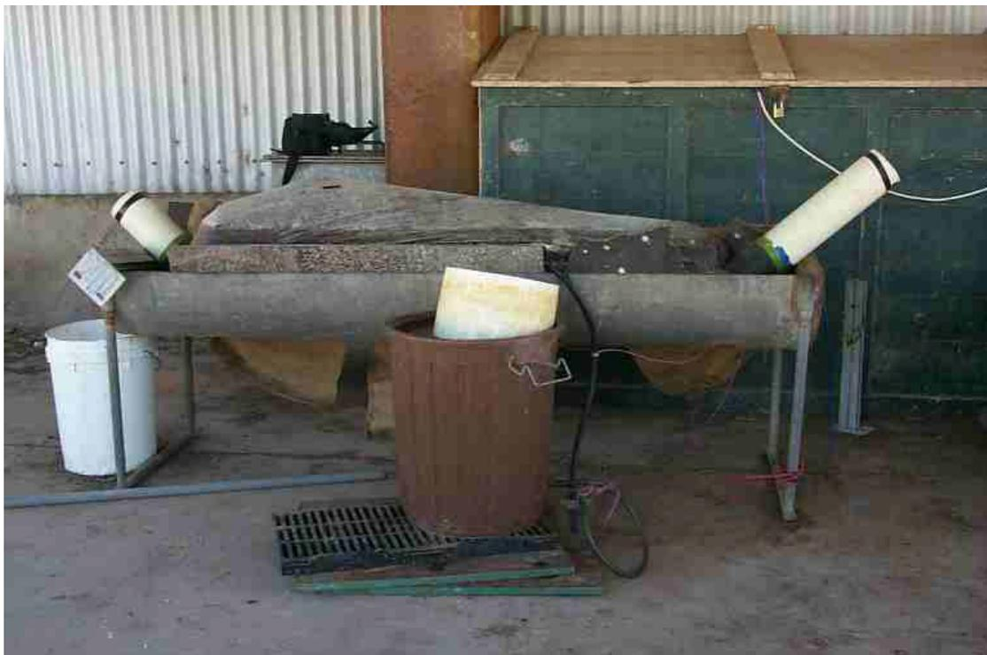
**Photograph 1 Demonstration poly Plug Flow Digester - Initial setup**
