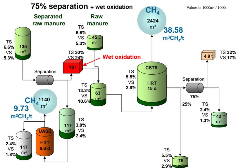
**Figure 6** Mass flow, methane yield and methane productivity for the system of manure separation combined with wet oxidation of the solid fraction
