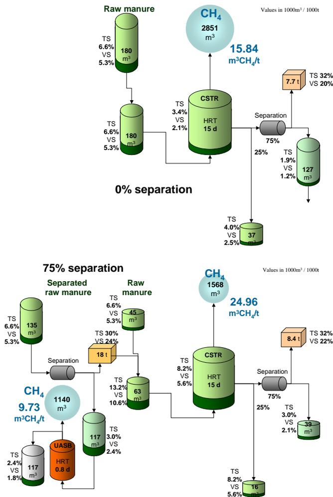
**Figure 4** Mass flow, methane yield and methane productivity for the system of manure separation (below) compared to the conventional system without separation(above)
