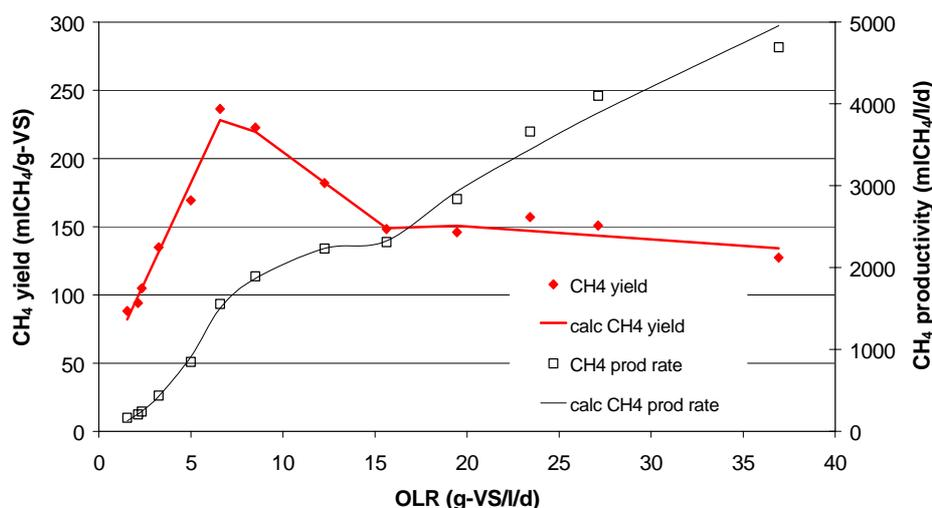
**Figure 3** Methane yield and productivity versus organic loading rate in UASB reactor
