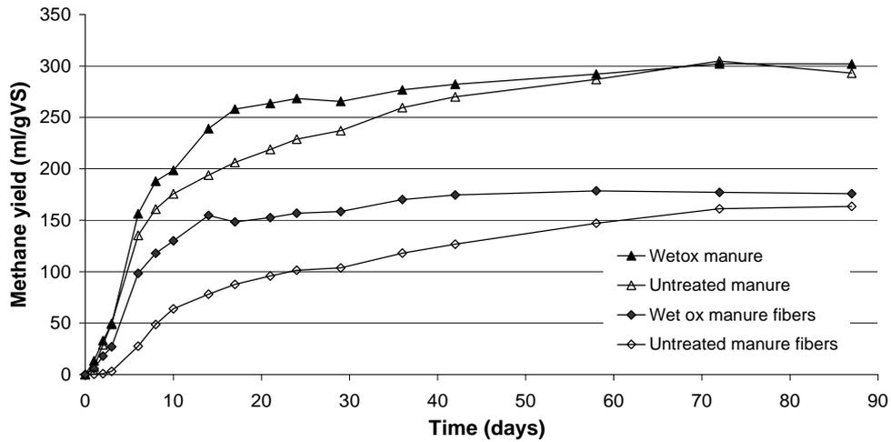
**Figure 5** Biogas potential before and after wet oxidation of unseparated cow manure and of manure fibers
