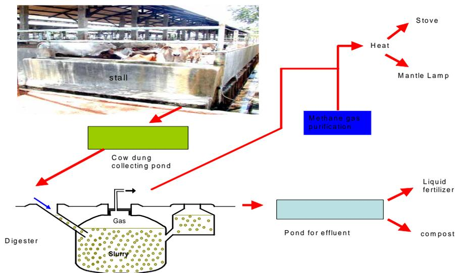
Figure 1. Schematic flow of Biogas Processing
